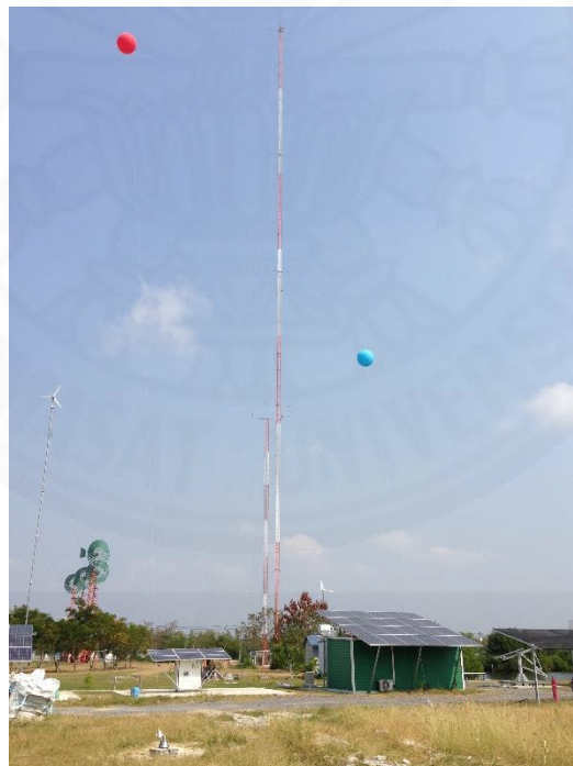
Figure 5.5 Determination of ground friction coefficient by using two sets of measurement device.
