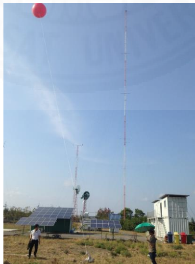
Figure 4.1 Experimental setup of wind measurement system using helium balloon near wind mast
