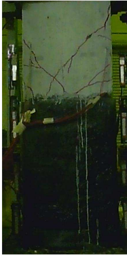
Figure 12-26: Failure mode of column FSD-CARB at 9% lateral drift
