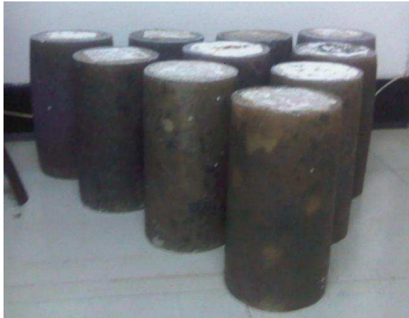
Figure 6-7: SFRP strengthened circular columns
