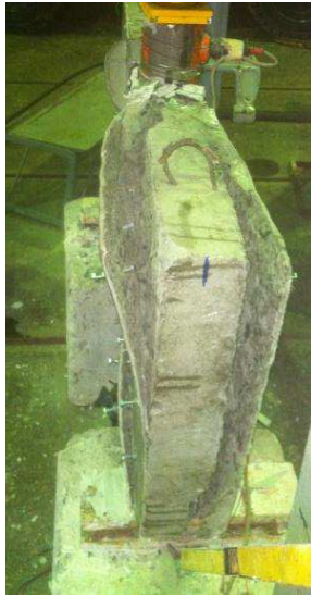
Figure 9-19: Failure mode of SGFRP strengthened beam specimen - HS-7A-S12
