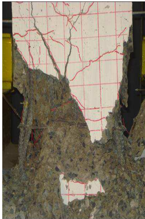
Figure 12-27: Failure mode of column FD-CON at 4.5% lateral drift
