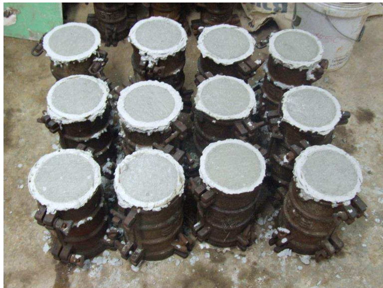
Figure 6-2: Preparation of circular columns
