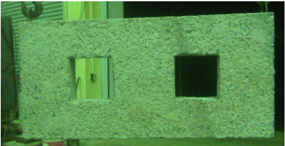
Figure 9-5: Roughened surface of concrete beam
