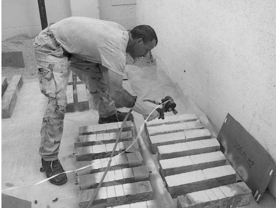
Figure 2-6: SFRP application in notched beams
