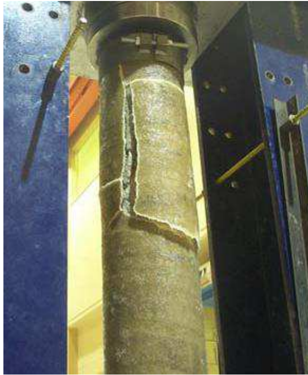
Figure 2-10: Failure of SFRP strengthened RC column
