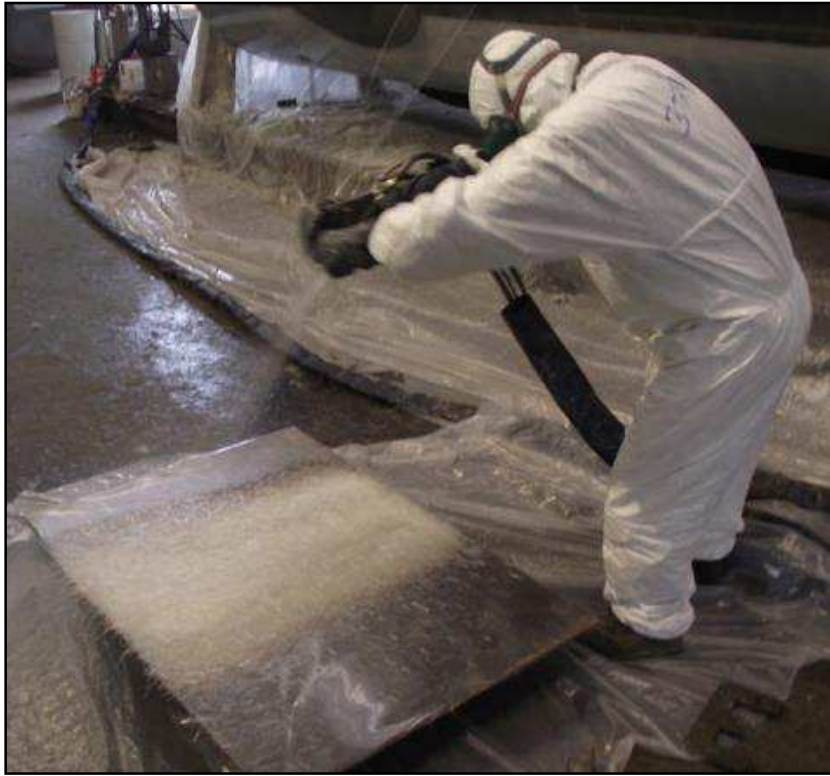
Figure 5-2: Spray process to prepare SFRP sheets
