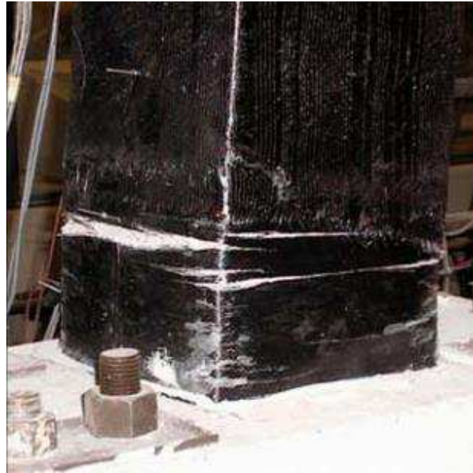
Figure 12-48: Rupture of FRP strap in hoop direction in FRP strengthened RC Column [34]
