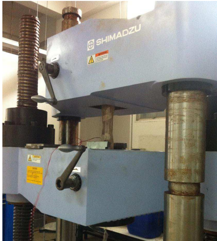
Figure 5-4: Loading setup to test SFRP tensile strips
