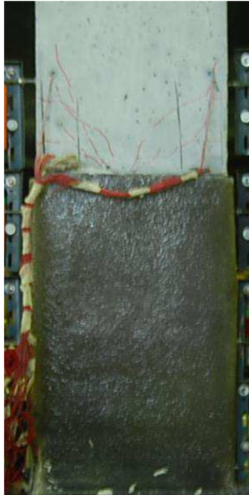
Figure 12-24: Failure mode of column SD-GLAS at 9% lateral drift
