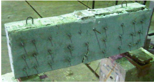
Figure 8-15: Failure mode of beam BN-LS-5GA-EB
