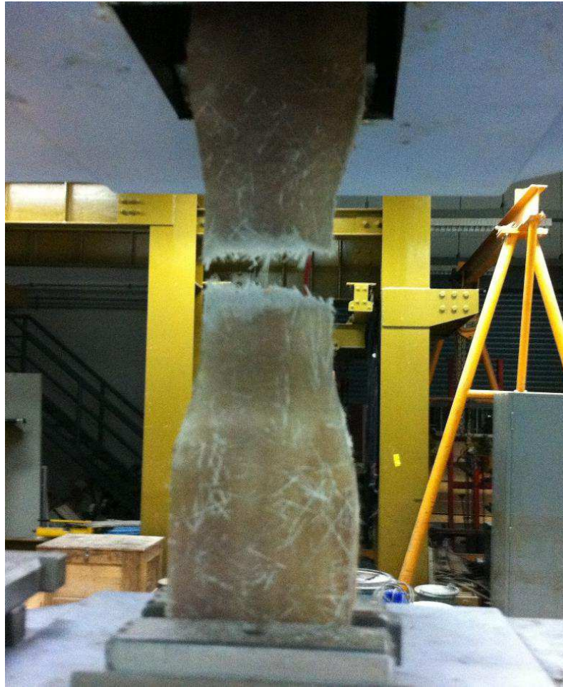
Figure 5-5: Typical failure of SFRP tensile strip
