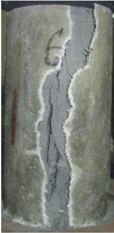
Figure 2-12: Typical failure of SFRP strengthened column
