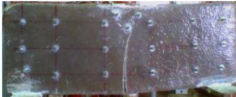
Figure 8-17: Failure mode of Beam BN-LS-5GA-MB2
