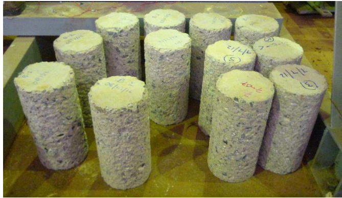
Figure 6-3: Column specimens with rough surface
