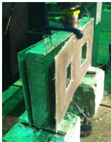
Figure 9-15: Failure mode of SGFRP strengthened beam specimen - LS-5A-S18-N
