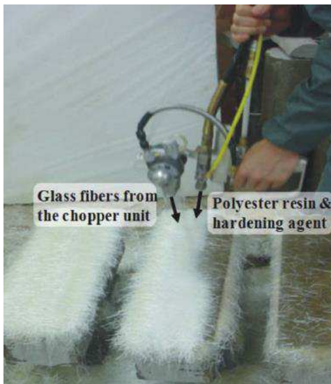
Figure 2-1: SFRP application to beam specimens
