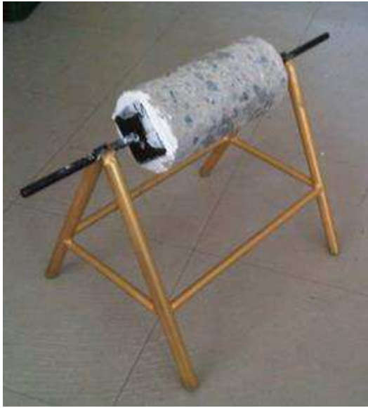
Figure 6-4: Arrangement for SFRP spray process
