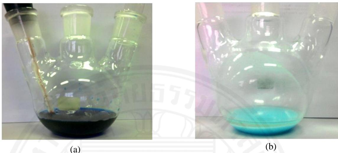
**Figure 3.3** Sol-gel preparation methods a) before sol-gel formation, b) after sol-gel formation
