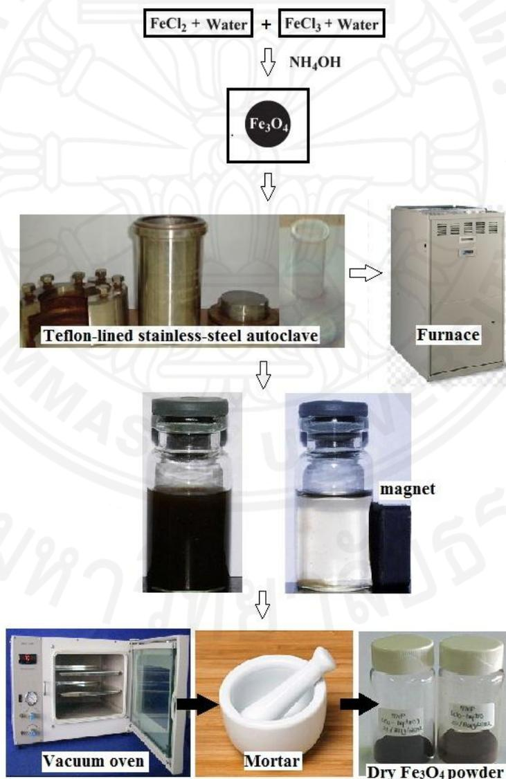
**Figure 3.2** Synthesis procedures of  $\text{Fe}_3\text{O}_4$  using co-precipitation, followed by hydrothermal treatment.
