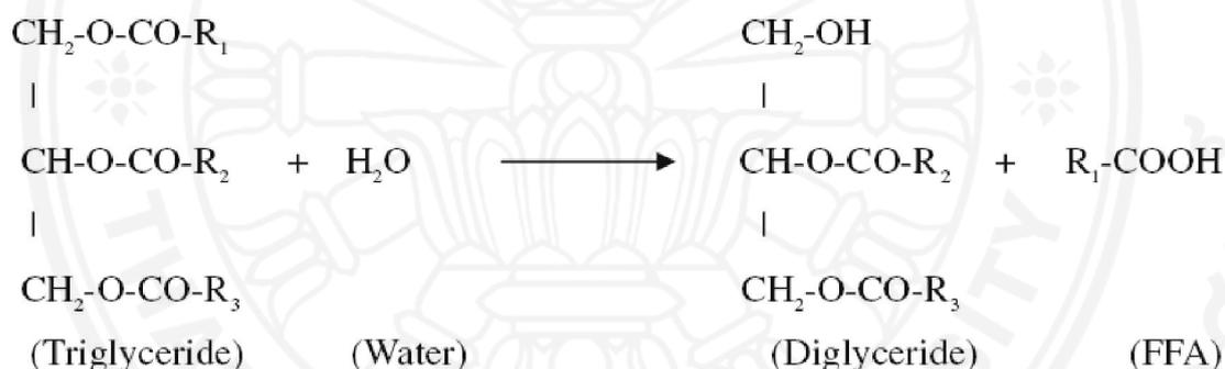
**Figure 2.6** The hydrolysis of triglyceride to form more undesirable FFA [13].
