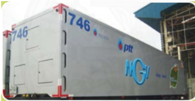
Figure 5.5 Neo Gas 2 Axels 9 Cylinders, Capacity 4 Tons per Trip
