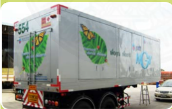
Figure 5.2 Semi-Trailers 80 Multi Cylinders, Capacity 2 Tons per Trip
