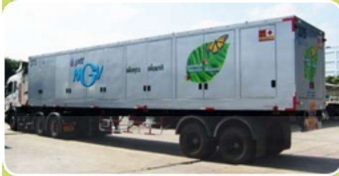
Figure 5.4 Long Tube Trailers 8 Cylinders, Capacity 3.2 Tons per Trip
