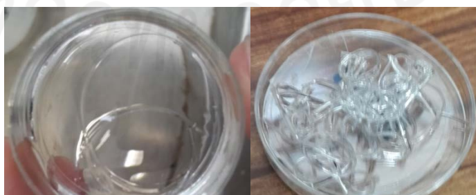
Figure 4.5 Thermal polymerization PNIAM- co -AM grafted on PS 6 well plate formed a linear PNIAM- co -AM.
