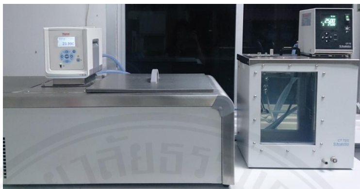
Figure 3.5: A temperature-controlled water bath and a viscometer chamber
