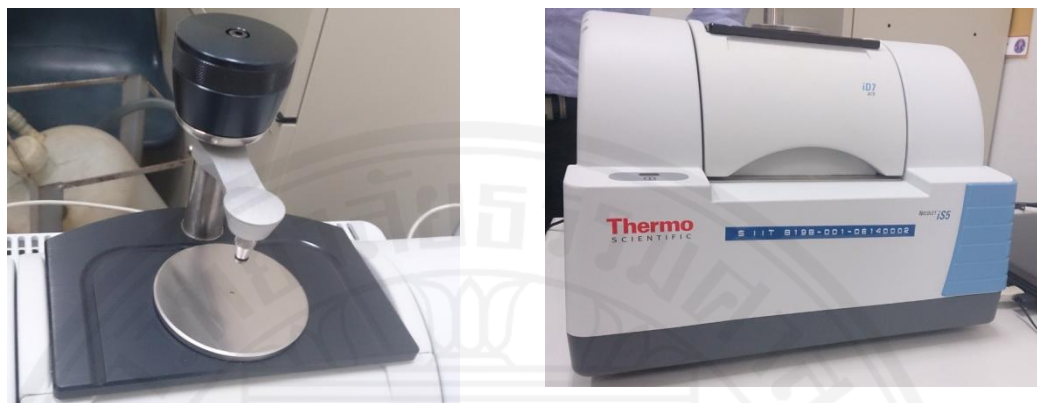
Figure 3.6: FTIR with a diamond ATR crystal (Single bounce technique)
