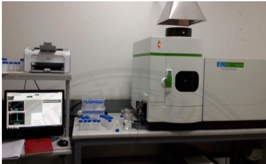
Figure 3.4: Heavy metals analysis by ICP-OES
