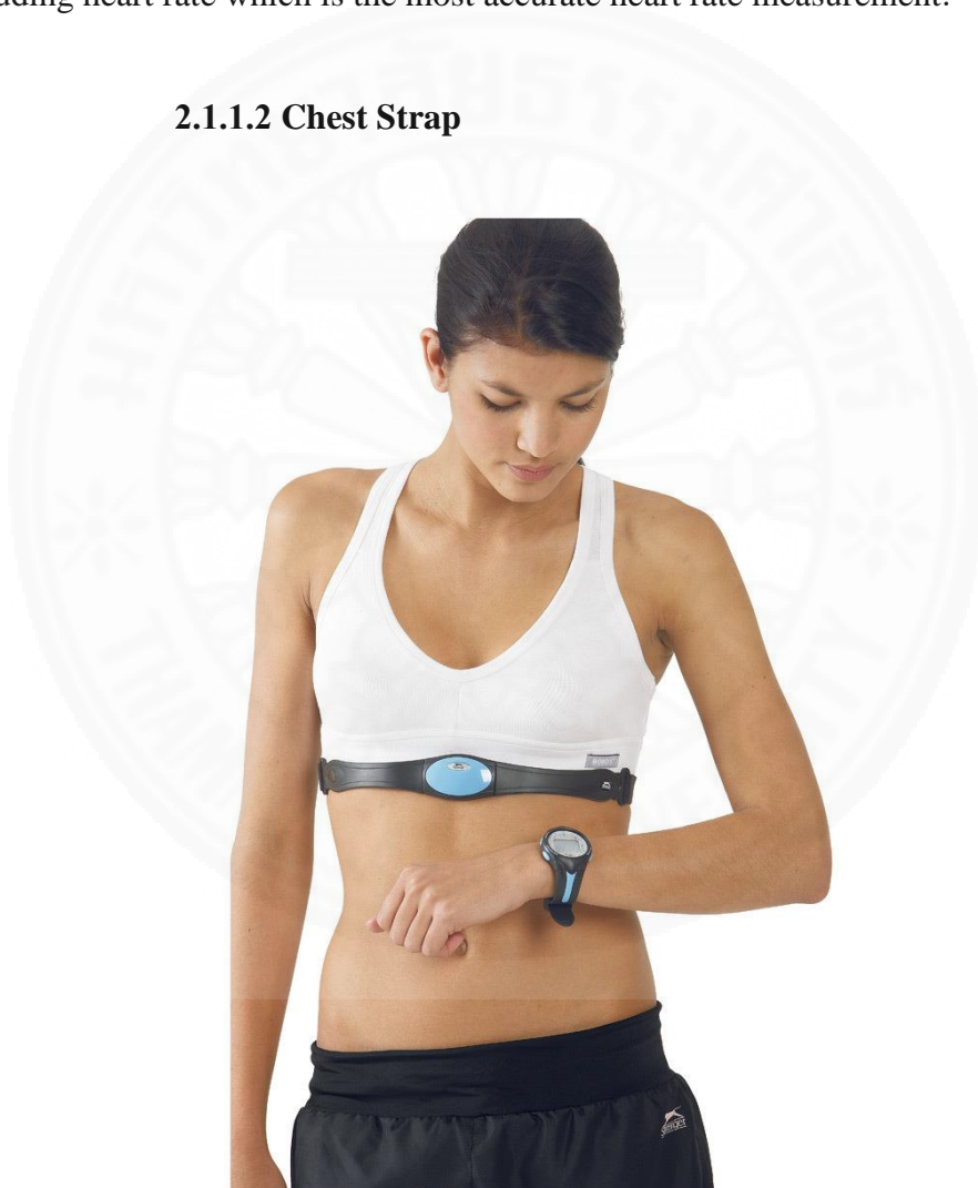
Figure 2.3: The image of chest strap heart rate monitor [15].
