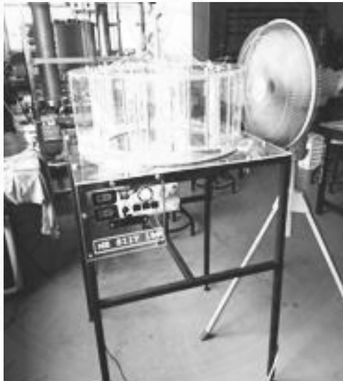
Figure 4.5 VAWT with wind booster during the experiment process
