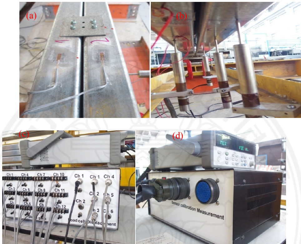
Figure 3.5. Detail of measurements : (a):Strain gauge; (b): LVDT; (c) (d): data logger
