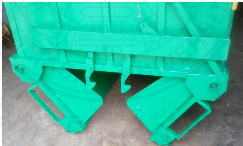
Figure 4 - 8. Checking mechanism of bottom door in reactor
