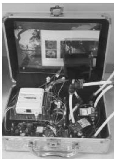
**Fig. 40a** The modified UV-Vis spectrophotometer “electronic nose”
