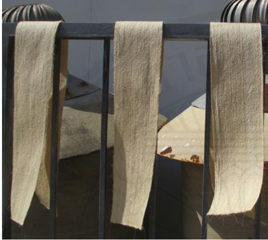
(a) Put Sisal fibers under sun light to make it fully dry at least 30 minutes.
