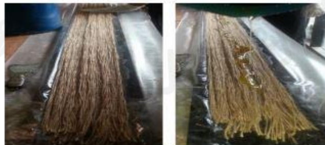
Figure 2.8 Fabricating of jute rope composite plate
