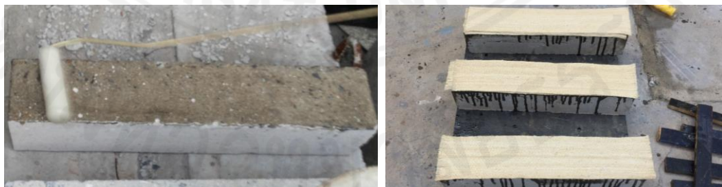
Figure 5.2 Hand layup process
