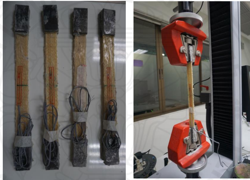
Figure 3.3 Tensile strength testing of hemp FRP composites
