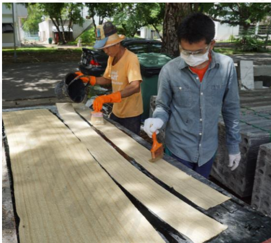
(c) Mix resin and apply on sisal fiber
