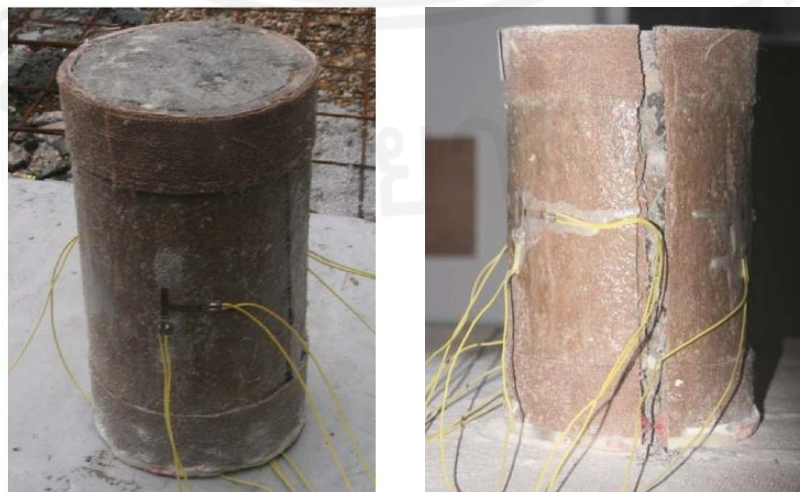
Figure 2.3 Cylinders wrapped by jute FRP
