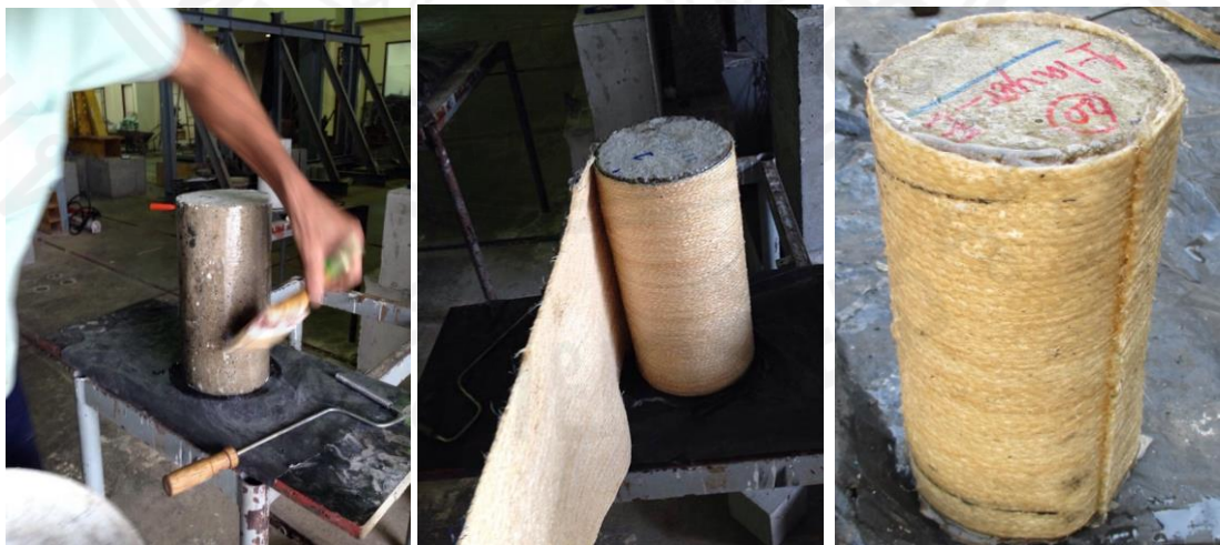
Figure 4.3 FRP wrapping procedure for cylindrical specimens
