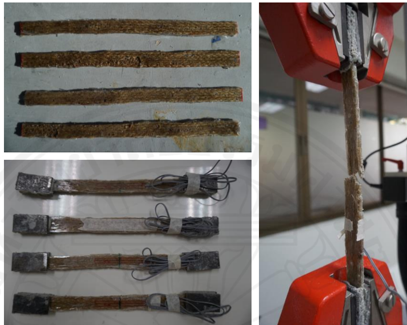
Figure 3.4 Tensile strength testing of hemp FRP composite
