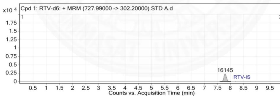
**Figure 4.5:** MRM Chromatogram of RTV-d6-IS: 500 ng/mL, (m/z 727.99->302.20)
