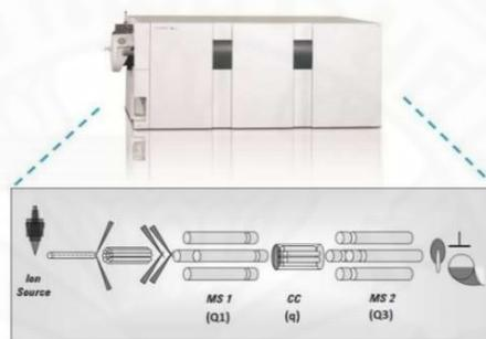
**Figure 3.5** Diagram of the Triple Quadrupole Mass Spectrometry System
