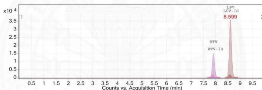
**Figure 4.1:** MRM chromatogram for lopinavir and ritonavir. RTV and RTV-d6-IS peaks were at 7.8 minutes; LPV and LPV-d8-IS peaks were at 8.5 minutes.
