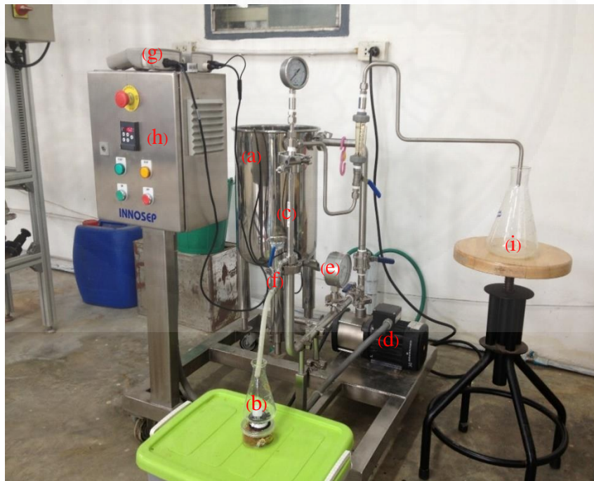
Figure 3.4 Picture of the bench-scale membrane test unit including: (a) feed tank, (b) permeate container, (c) membrane modules, (d) feed pump, (e) feed pressure gauge, (f) permeate flow meter, (g) pH and conductivity monitor, (h) control panel, and (i) retentate container
