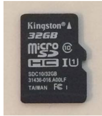
Figure 3.3 32 GB Micro SD card for Raspberry Pi2 module B
