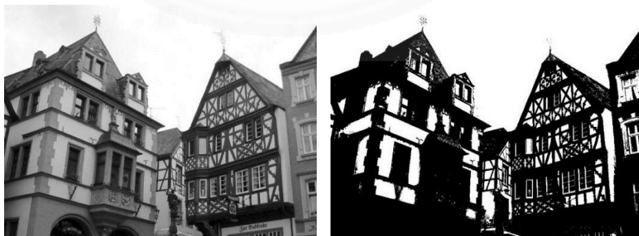
Fig. 2.5 Original grayscale image (left), Post-thresholding binary image (right) [21]
