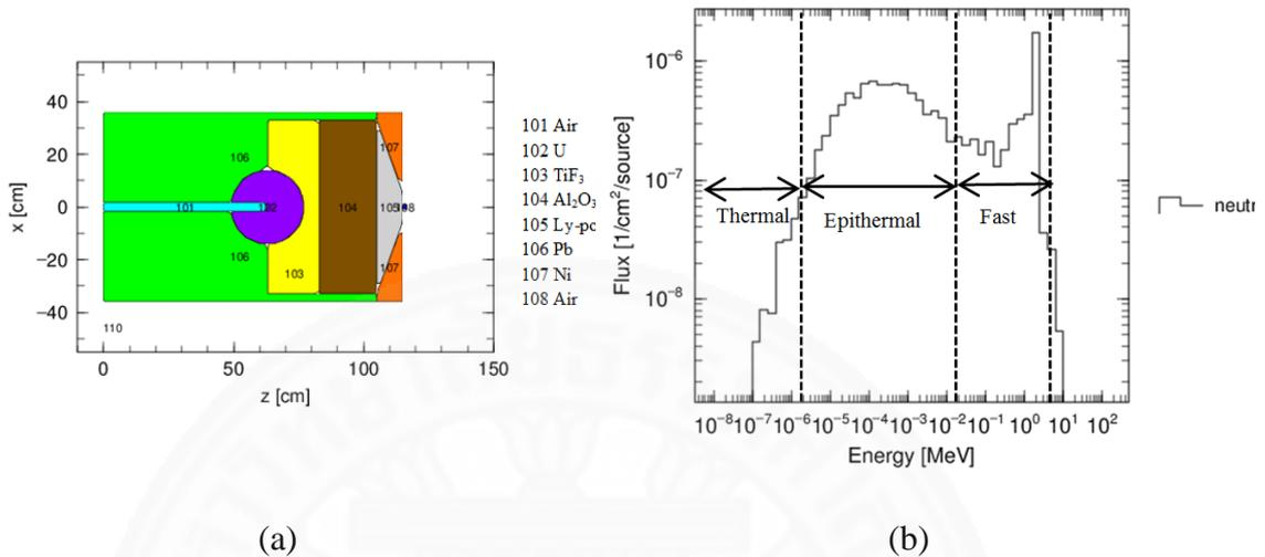
Figure 4. 7 The BSA design B (a) and neutron flux per neutron source at the beam port exit versus energy proposed (b). The BSA design was proposed by Rasouli and Masoudi (2012).
