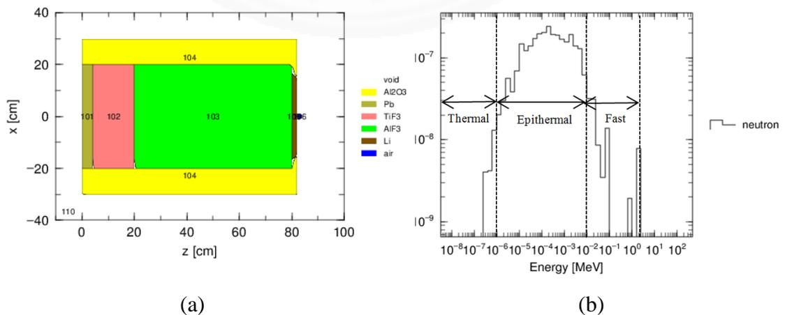
Figure 4. 5 The proposed BSA design (a) and the neutron flux per neutron source at the beam port exit versus neutron energy (b).
