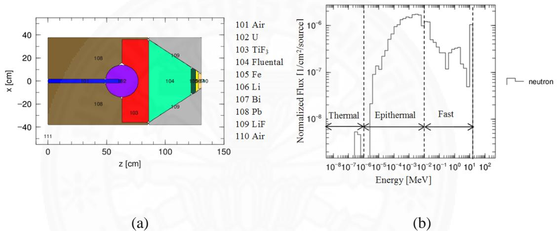
Figure 3. 3 The BSA design (a) and neutron beam port flux per neutron source versus energy (b) proposed by Rasouli et al. (Rasouli et al., 2012).
