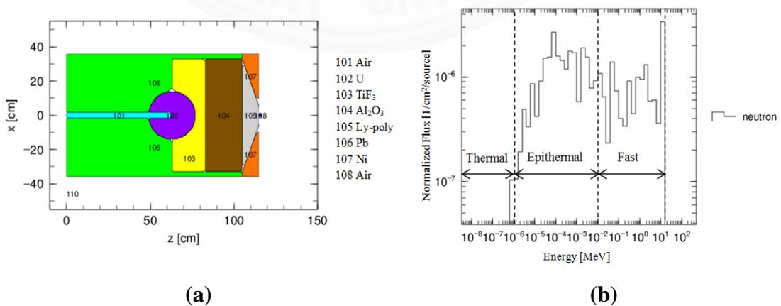
Figure 3.2 The BSA design (a) and neutron beam port flux per neutron source versus energy proposed (b) proposed by Rasouli and Masoudi (Rasouli & Masoudi, 2012).
