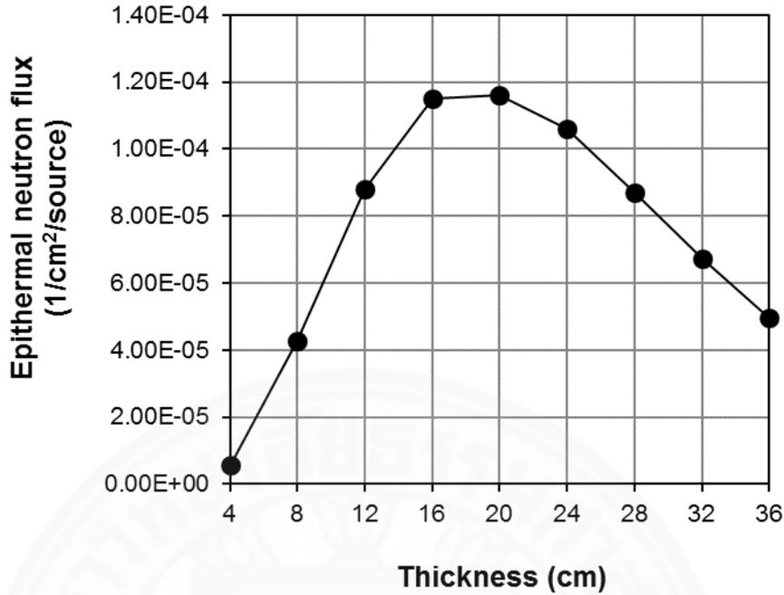
Figure 4. 2 Epithermal neutron flux per neutron source for different thicknesses of TiF<sub>3</sub> as the first moderator
