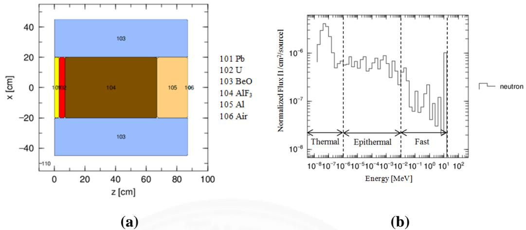
Figure 3. 1 The BSA design (a) and neutron beam port flux per neutron source versus energy (b) proposed by Eskandari and Kashian (Eskandari & Kashian, 2009).
