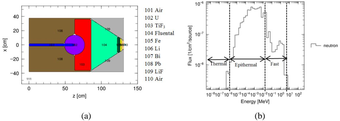
Figure 4. 8 The BSA design C (a) and neutron flux per neutron source at beam port exit versus energy (b). The BSA design was proposed by Rasouli et al. (2012).
