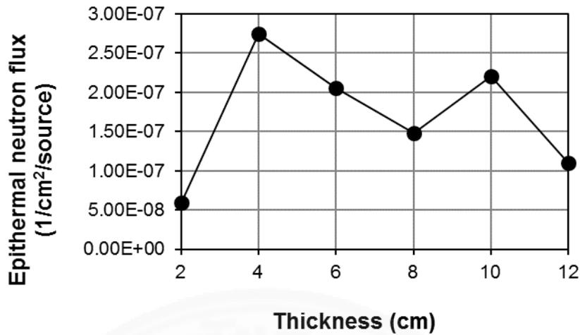
Figure 4. 1 Epithermal neutron flux per neutron source for different thicknesses of Pb as the multiplier.
