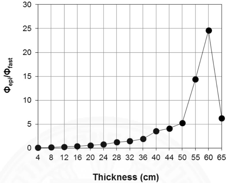
Figure 4. 3  $\phi_{epi}/\phi_{fast}$  for different thicknesses of  $AlF_3$  as the second moderator.
