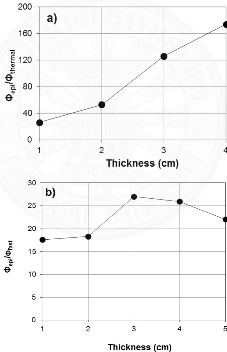
Figure 4. 4  $\phi_{\text{epi}}/\phi_{\text{thermal}}$  (a) and  $\phi_{\text{epi}}/\phi_{\text{fast}}$  (b) for different thicknesses of Li as the thermal neutron filter.
