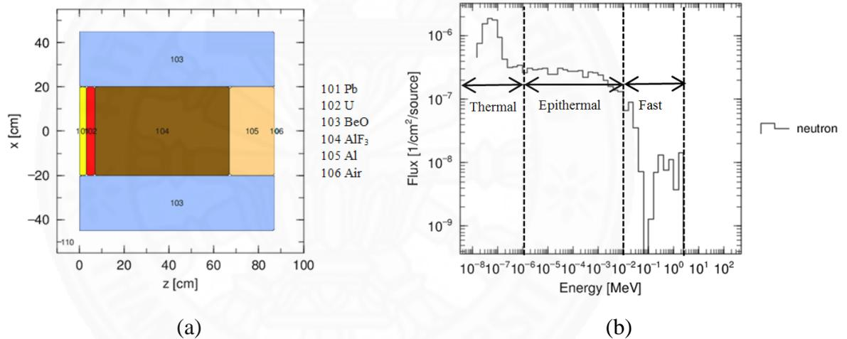
Figure 4. 6 The BSA design A (a) and the neutron flux per neutron source at the beam port exit versus energy (b). The BSA design was proposed by Eskandari and Kashian (2009).
