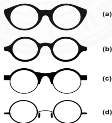
Figure 6.2: Various frame styles of the circular shapes of eyewear; (a) fashionable frame, (b) full-plastic frame, (c) semi rimless, and (d) full-metal frame
