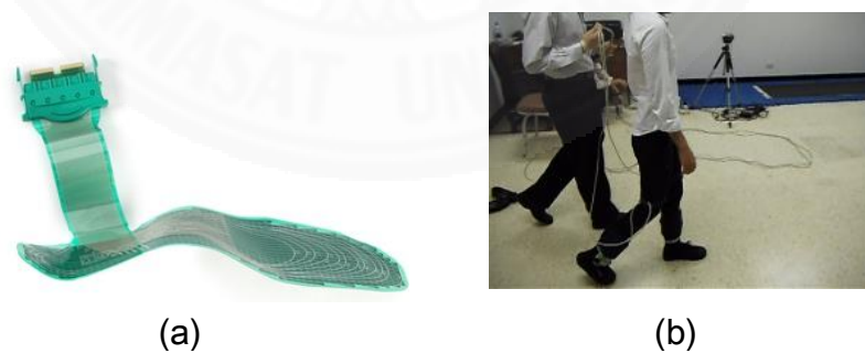
Figure 4.5: Tek-Scan simulation: (a) Flexible, thin-in shoe load cell, (b) The experimental conducting for walking
