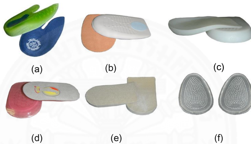
Figure 4.4: Six types of heel insoles: (a) specimen 1 (gel and rubber with cloth on top), (b) specimen 2 (natural latex foam), (c) specimen 3 (silicone gel), (d) specimen 4 (gel with cloth on top), (e) specimen 5 (soft foam), (f) specimen 6 (invisible gel)
