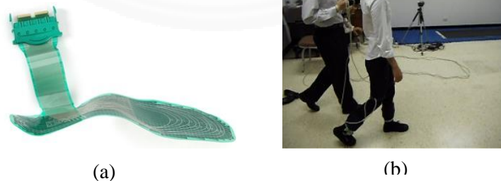
Figure 3.16: Tek-Scan simulation: (a) Flexible, thin-in shoe load cell, (b) The experimental conducting for walking
