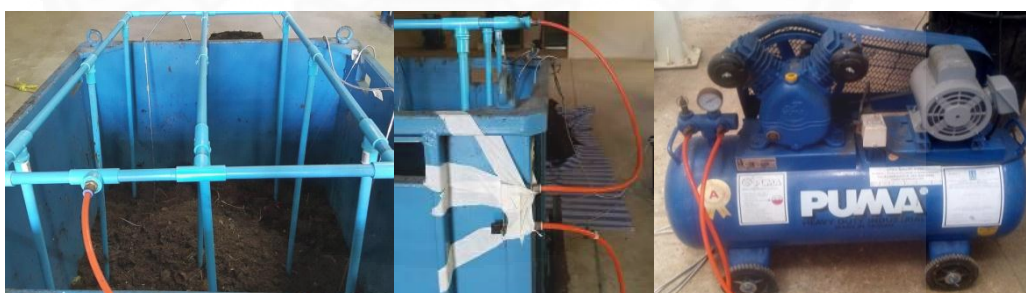
Figure 3.24 Setting up of aeration system
