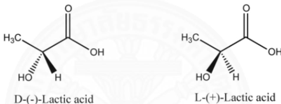
**Figure 2.14** Chemical structure of lactic acid isomers (Garrison et al., 2016).
