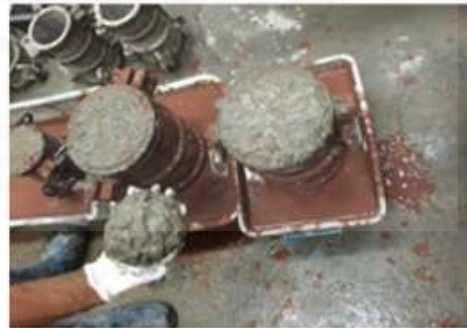
b) A concrete sample in the mould containing bentonite fluid
