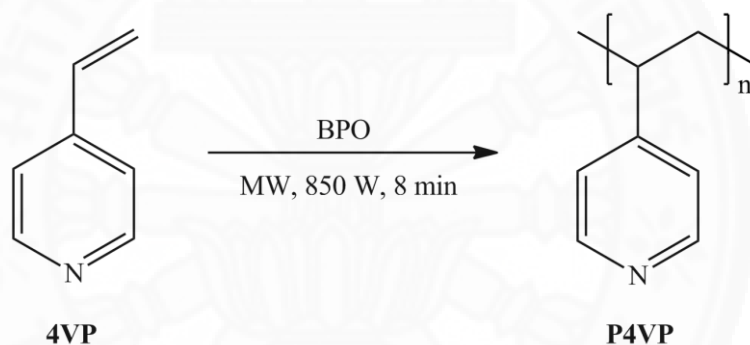
Figure 20 Synthesis of poly(4-vinylpyridine) from 4-vinylpyridine (4VP) and benzoyl peroxide (BPO) as a monomer and initiator, respectively.
