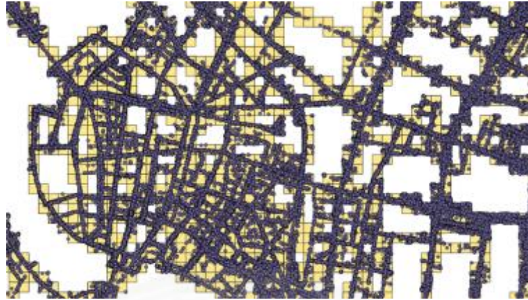
Figure 3.2: The road segment which we map to grid 100 meters
