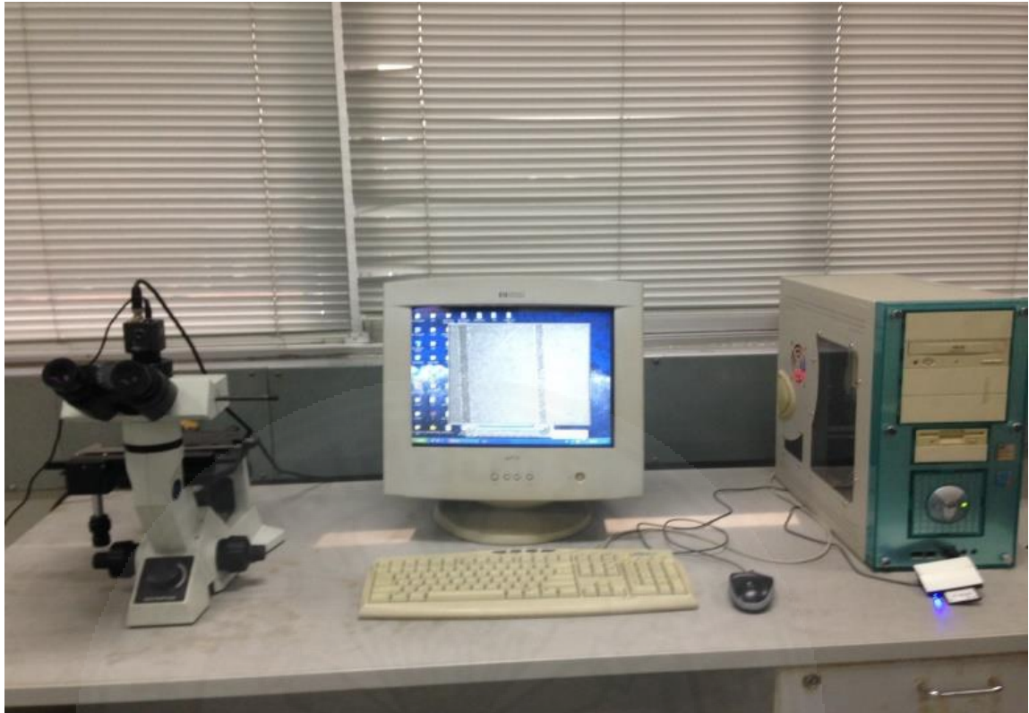
Figure 3.12 Microscope scanning device with 10x, 20x, 50x and 100x magnification.
