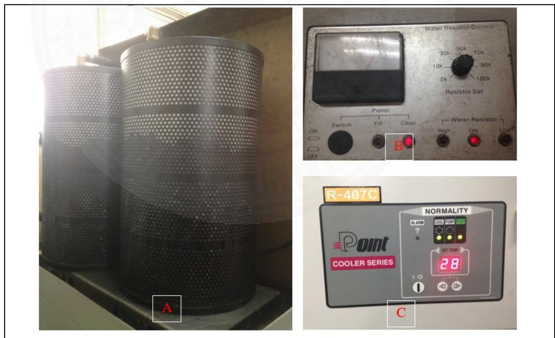
Figure 3.7 (A) Resin pump, (B) Dielectric conductivity meter and (C) Temperature controlling device
