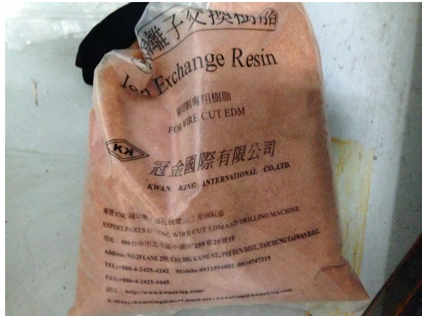
Figure 3.6 Ion exchange resin for wire-EDM dielectric
