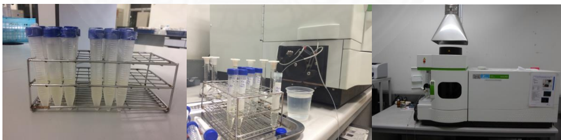
Figure 3.5 Steps for analyzing residual lead concentration in the sample using an Inductively Coupled Plasma (ICP) Spectrometer
