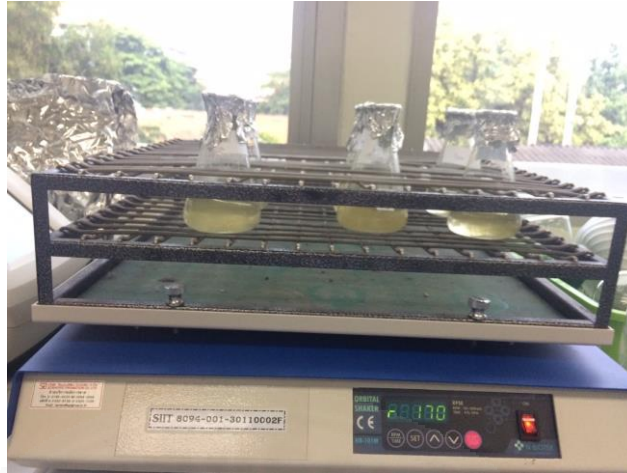
Figure 3.3 Adsorbent samples with lead solution were shaken in the rotary shaker
