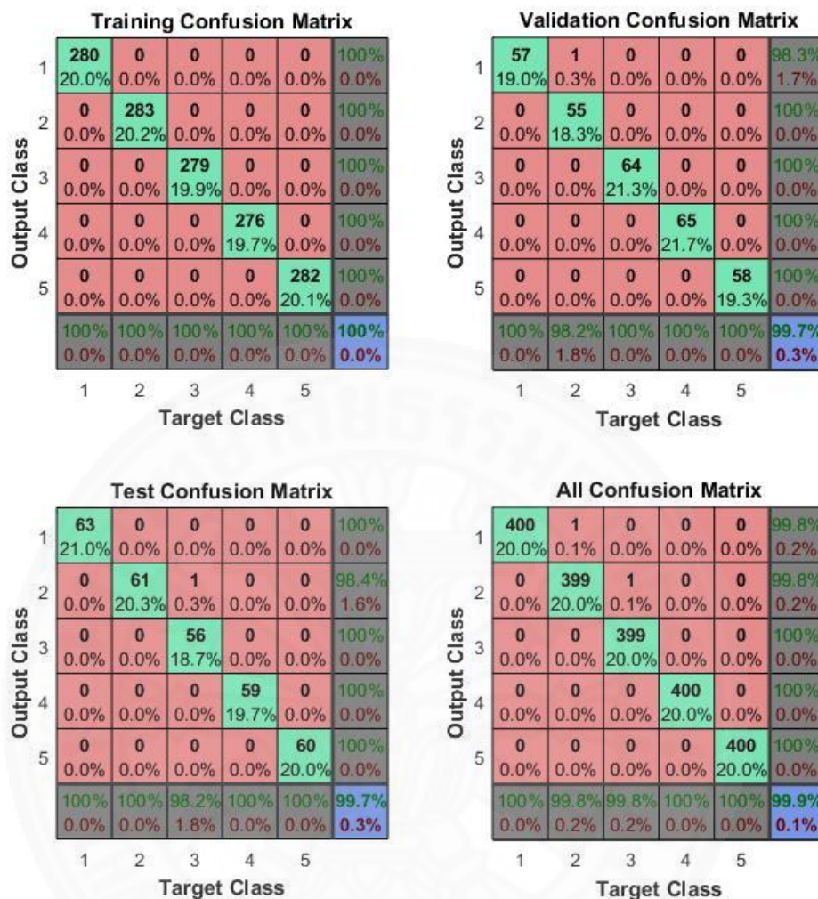
Confusion matrix of posture classification using 120 inputs with normalized signal data of subject A
