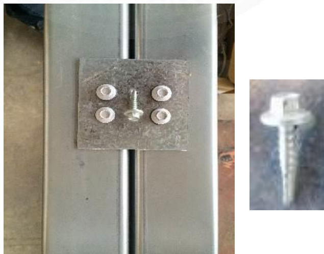
Figure 3.2 Stiffening plate (80x80x2mm) with 4 screws
