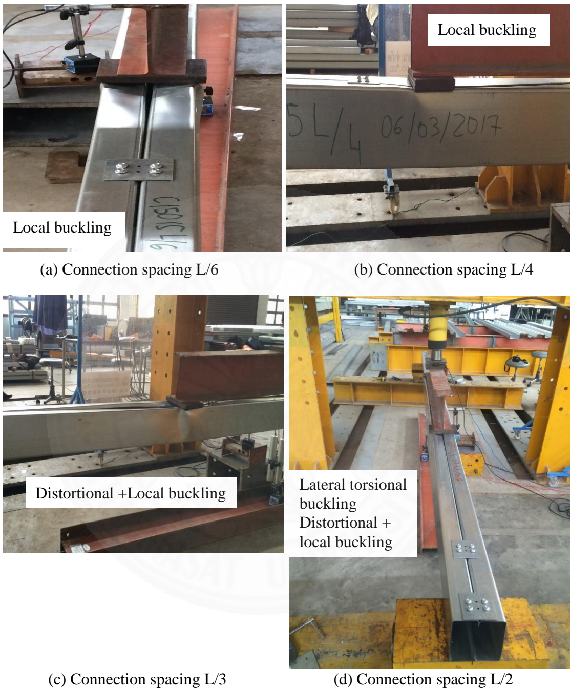
Figure 3.28 Failure mode of BBC-15015
