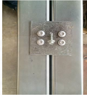
Figure 1.9 Screw connection with stiffening plate used in this thesis (80x80x2mm)
