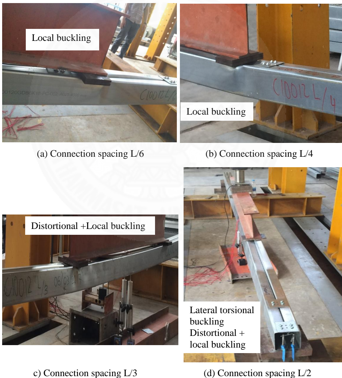
Figure 3.24 Failure mode of BBC-10012
