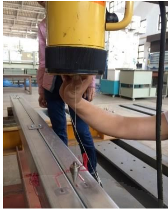
Figure 3.8 Checking the centerlines
