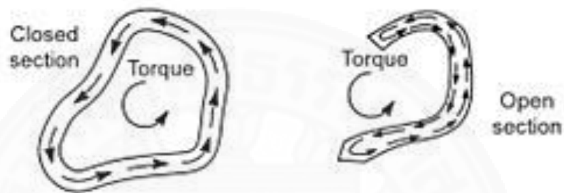
Figure 1.6 Torsion of closed and open thin-walled section
