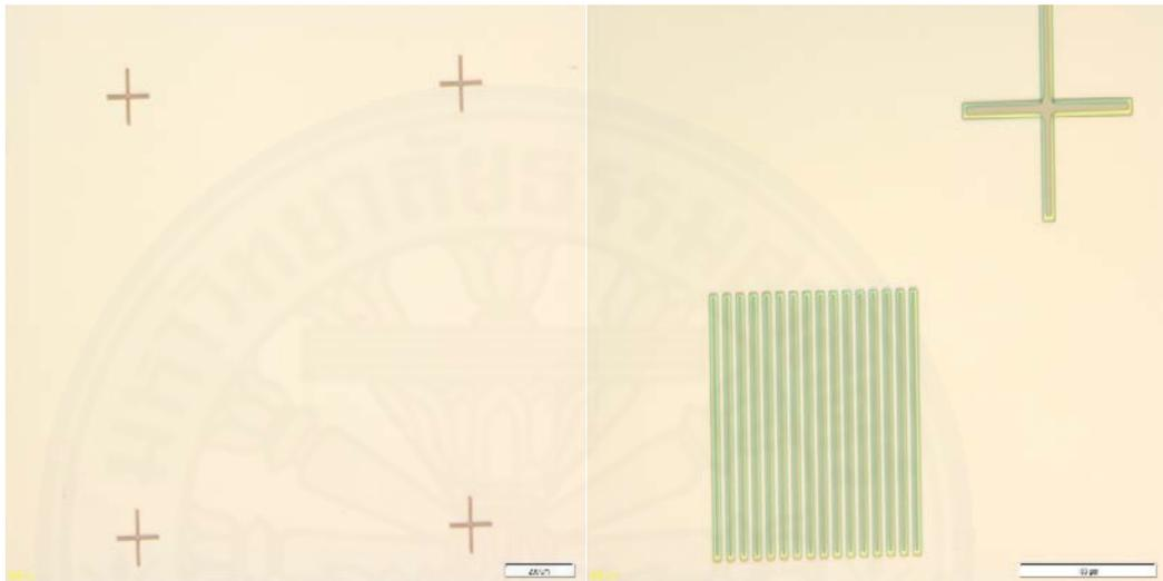
Figure 5.4 After developing the PR, the pattern mark is clean, completed develop.
