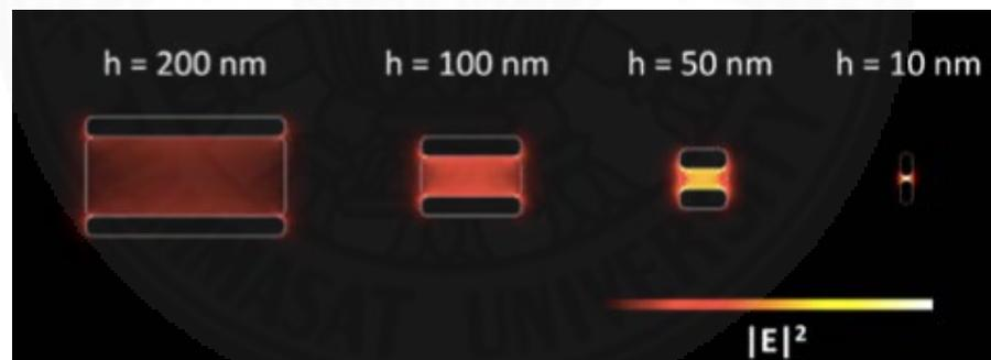
Figure 2.12 Cross-sectional side views of the  $E^2$  profiles along the  $y$ - $z$  plane for  $h = 200, 100, 50,$  and  $10 \text{ nm}$ , respectively [57].
