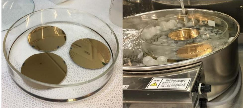
Figure 5.7 (Left) NMP lift-off process for one night and (Right) after one night will add more temperature for complete lift-off remove.
