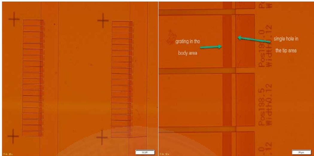
Figure 5.54 Microscope observation of the 130 nm-thickness of PR after developed by GL2000 developer (Xylene) 90 s and rinse by GL-2000 Rinse (IPA)
