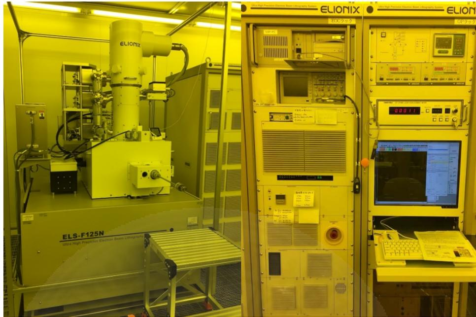
Figure 5.52 The ultra-high precision electron beam lithography system (E-Beam lithography)
