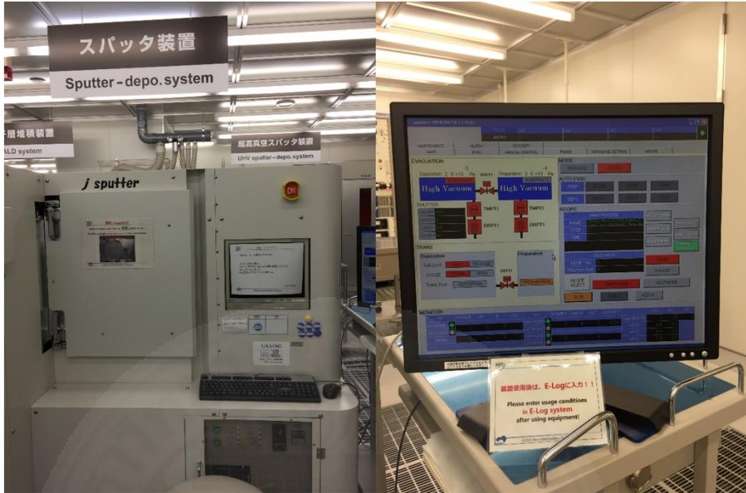
Figure 5.5 The J sputter and monitor for controlling operate to sputter Au-Ti-SiO<sub>2</sub> Film.
