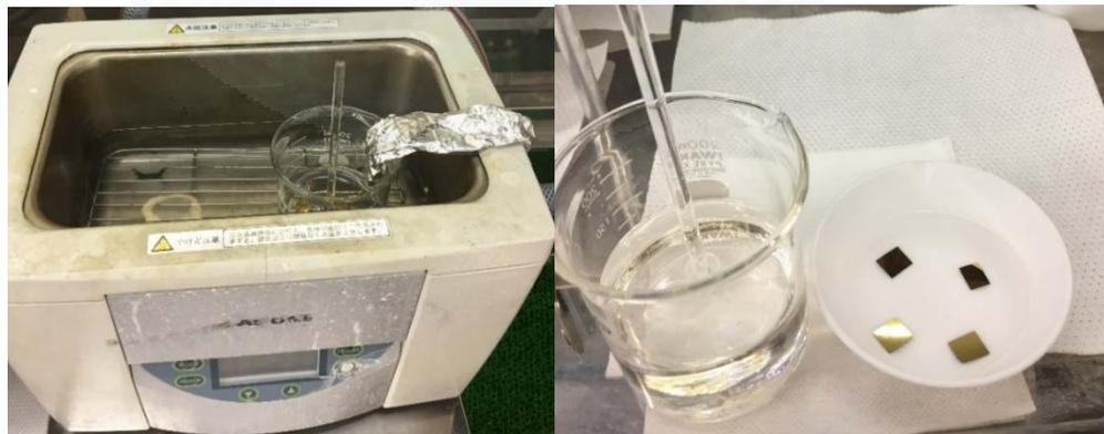
Figure 5.45 NMP sonication, acetone, and IPA cleaning.
