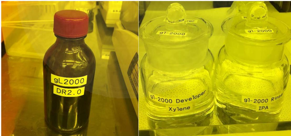
Figure 5.64 (Left) GL2000 DR 2.0 EBeam-Photoresist and (Right) GL2000 Developer
