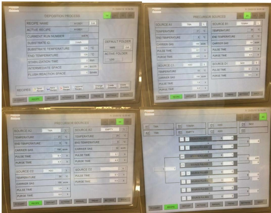
Figure 5.49 The recipe of ALD of the 40 nm-thickness Al<sub>2</sub>O<sub>3</sub>.
