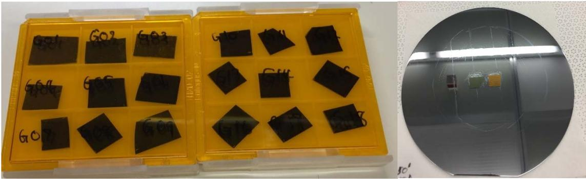
Figure 5.29 (Left) 'G'-pure 200 nm-SiO<sub>2</sub> thickness, (Right) Small piece of 'G' wafer and our sample for etching in the same condition.
