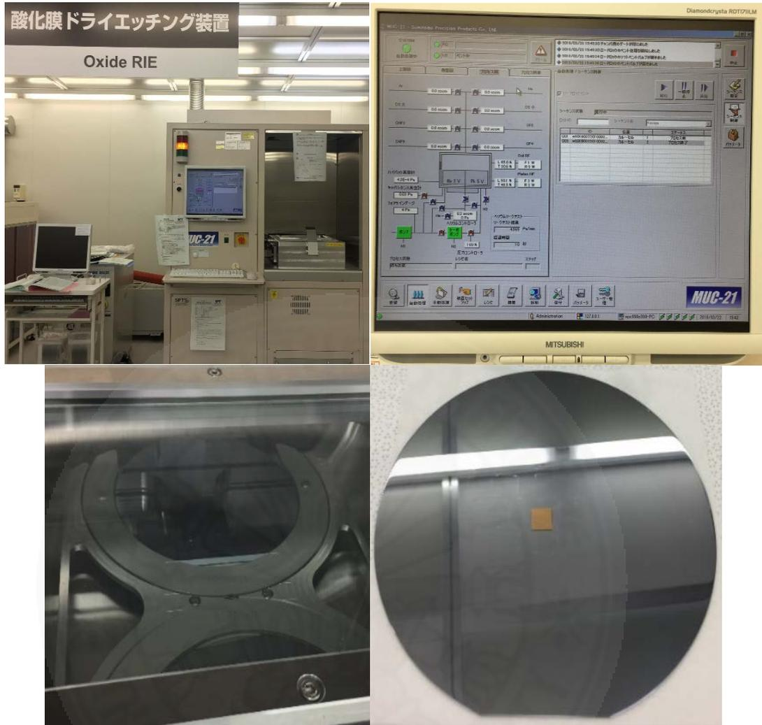
Figure 5.16 Oxide Dry Etching machine, user interface, Dry etching tray for loading the sample, and the sample preparation on dry etching holder.
