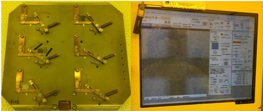
Figure 5.67 (Left) the holder of the E-Beam lithography with 'A' and 'B' specimens (Right) the mask for origin point adjustment.
