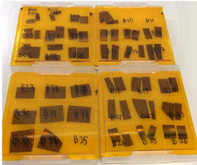
Figure 5.35 The actual sample after dry etching process
