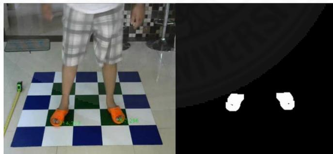
Figure 3.2 HSV Color Thresholding
