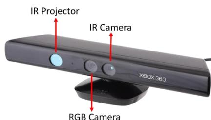
Figure 2.2 Microsoft Kinect Sensor
