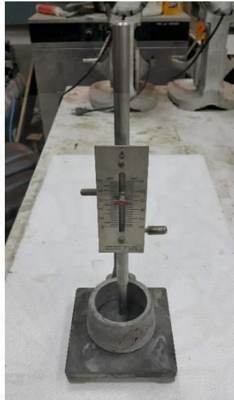
Figure 3.4 Apparatus for testing setting time of paste
