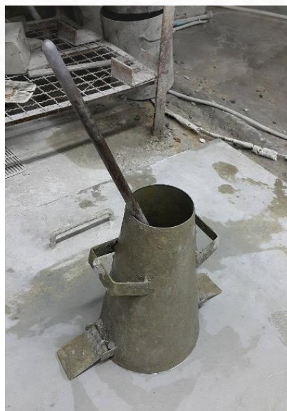
Figure 3.6 Apparatus for slump test
