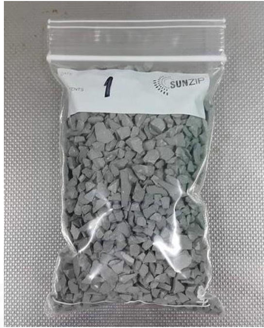
a) Sieved specimen with size between 2.36-4.75 mm
