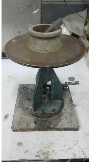
Figure 3.5 Apparatus for testing water requirement
