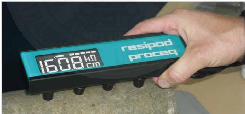
Figure 2.11 Commercially available Wenner probe
