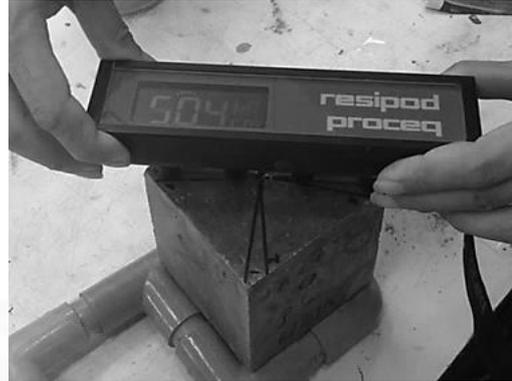
Figure 3.3: Measurement technique for electrical resistivity of a cubic specimen using a four Wenner probe
