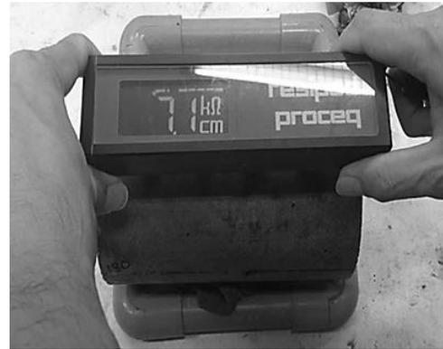
Figure 3.5: Measurement technique for electrical resistivity of a cylindrical specimen using a four Wenner probe
