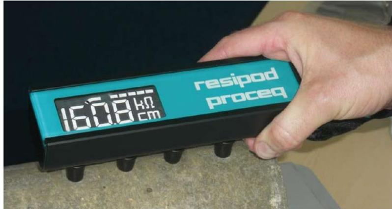
Fig 1.2 Surface resistivity meter (four Wenner probe)
