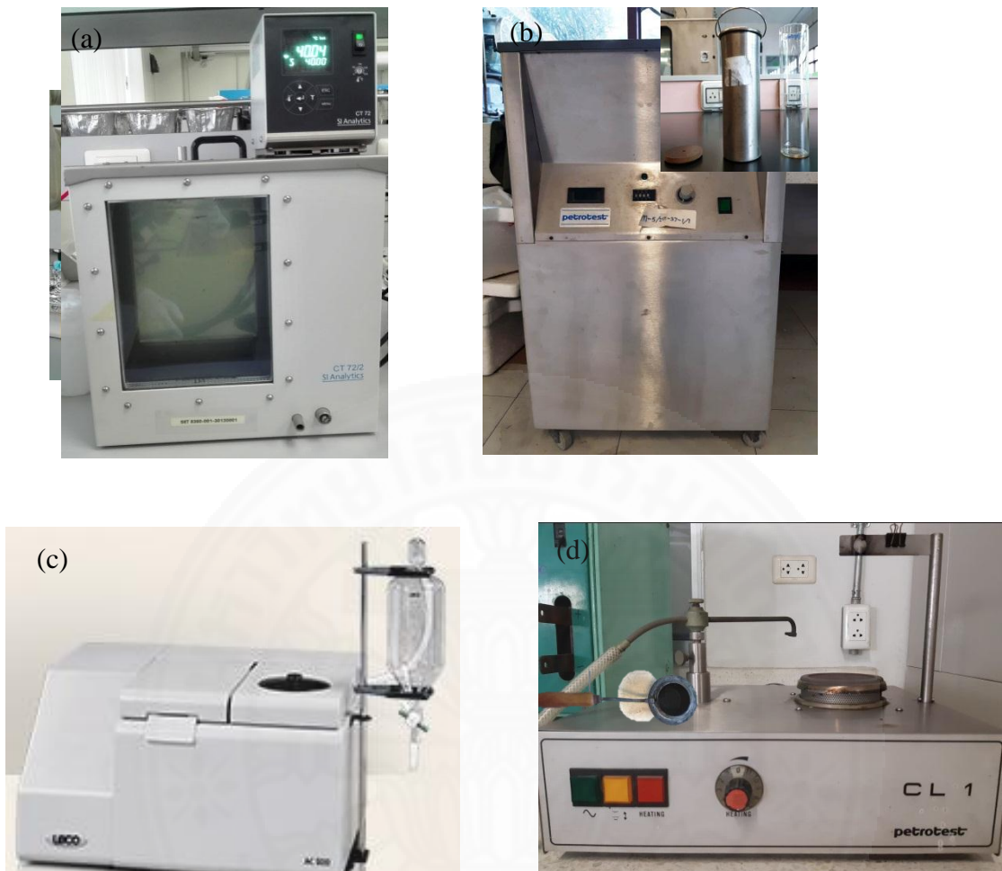
Fig. 4B Experimental setups used for biodiesel characterization (a) viscometer, (b) pour point tester, (c) bomb calorimeter, (d) open-cup flash point tester
