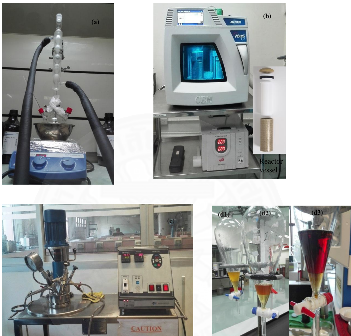
Fig. 3B Biodiesel production (a) conventional open reflux reactor, (b) microwave reactor, (c) autoclave reactor, and (d) phase separation of biodiesel produced in (d1) autoclave reactor, (d2) microwave reactor, and (d3) autoclave reactor
