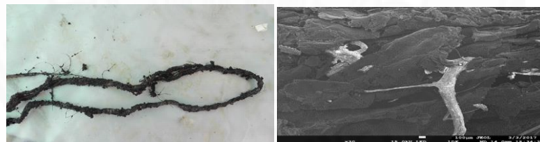
Figure 4.8 Naked eye view and SEM image of carbon fiber
