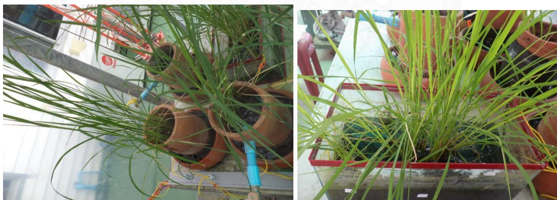
Figure 4.1 Lab-scale paddy microbial fuel cell: Double chamber(A), Single chamber (B)
