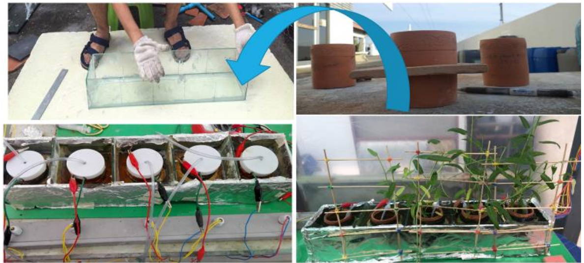
Figure 3.3 Fabrication of double chamber hydrophytes operated PMFC
