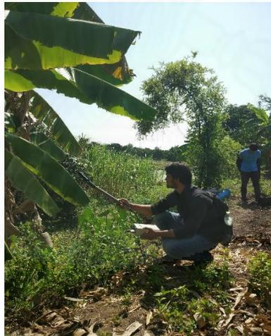
Figure 4.3: Field measurements with LI-COR LAI 2000 Plant Canopy Analyzer.
