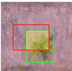
Figure 3.14: Object localization example, where the green polygon represents the ground labelled truth, while the red polygon represents the algorithm detected bounding box.
