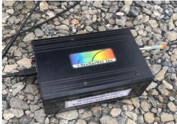
Figure 3.3: Spectrometer (Black Comet C-200 TEC ranging from 200-1100nm)
