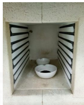
Carbonization in muffle furnace
