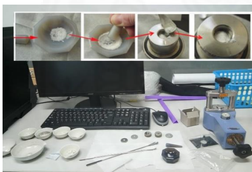
Sample preparation for FTIR in the manual bench press
