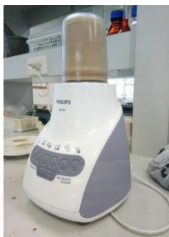
Grinding the adsorbents in powdered form
