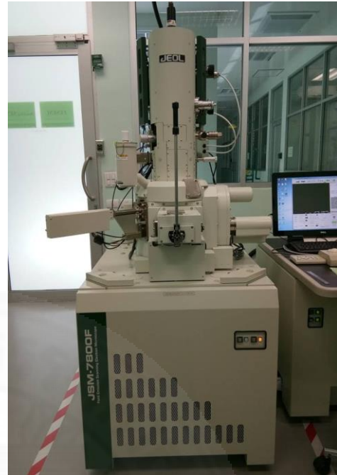
FESEM equipped with an EDX
