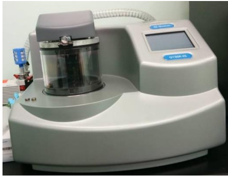
Instrument used to do gold coating
