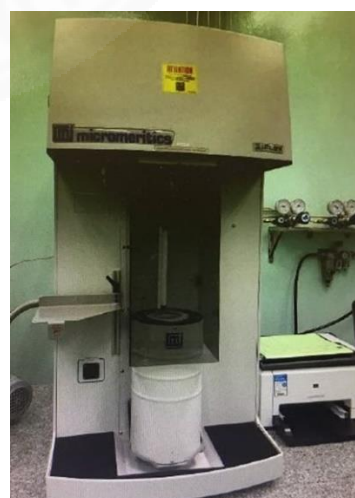
Flex (N 2 adsorption instrument used for surface area analysis)
