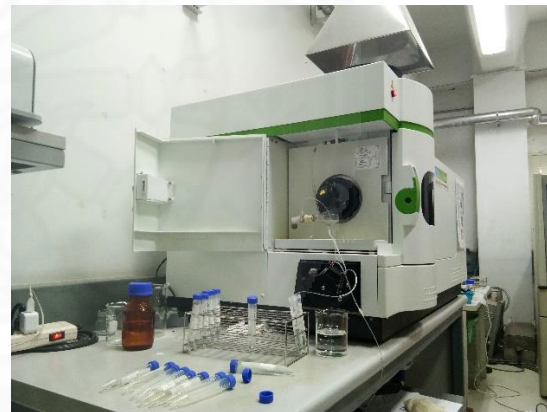
Arsenic measurement using ICP-OES
