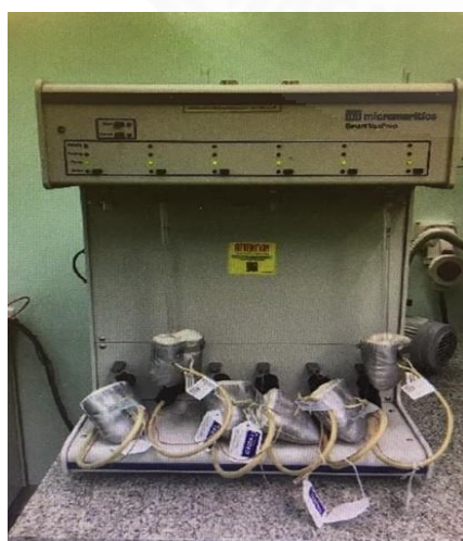
Smart vacuum (sample preparing instrument for surface area analysis).
