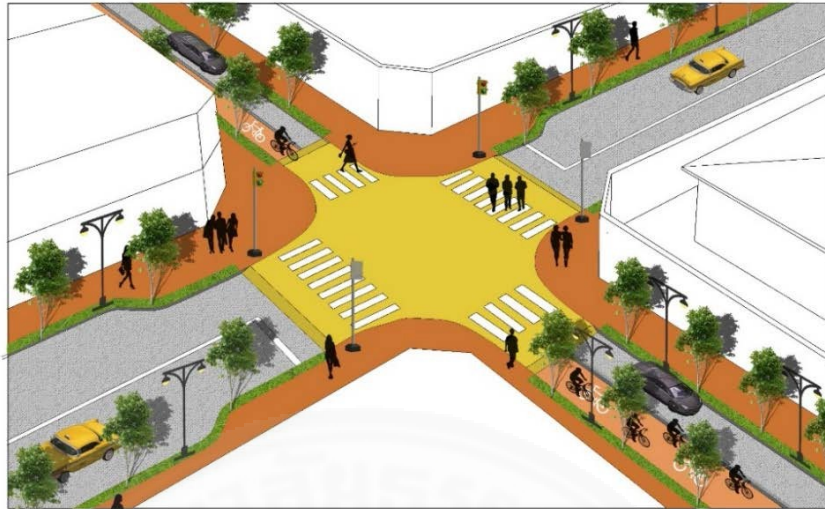
Figure 6.14 Raised intersection on Chaing Mai – Lamphun road
