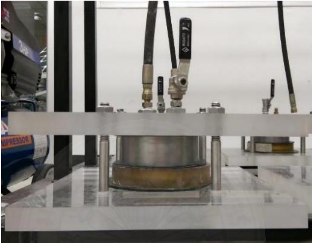
Figure 3.13 Install sample into water permeability cell.
