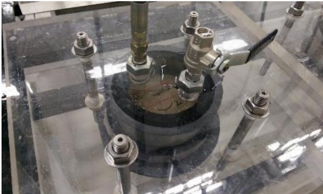
Figure 3.14 Fully fill water into the water permeability cell.
