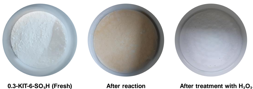
Figure 3.11 0.3-KIT-6-SO 3 H catalyst before and after regeneration
