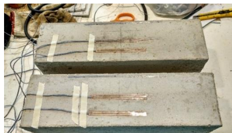
Figure 3.3 Prisms for tensile strain capacity test
