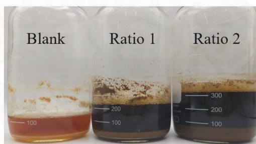
Figure 4.11 The preliminary experiment of vary sample concentration of 10, 20, 30 mL at \text{FeSO}_4 30 mg, \text{H}_2\text{O}_2 3 mL, reaction pH 4 at reaction time 24 hours
