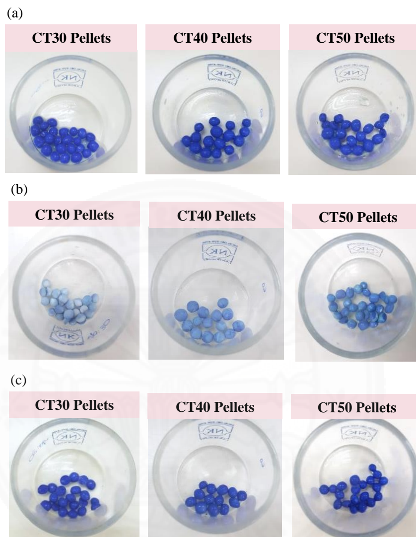
Figure 4.14. MB on clay TiO 2 pellets: (a) under dark condition for 90 mins (b) under UVA light for 240 mins and (c) under dark condition for 90 mins
