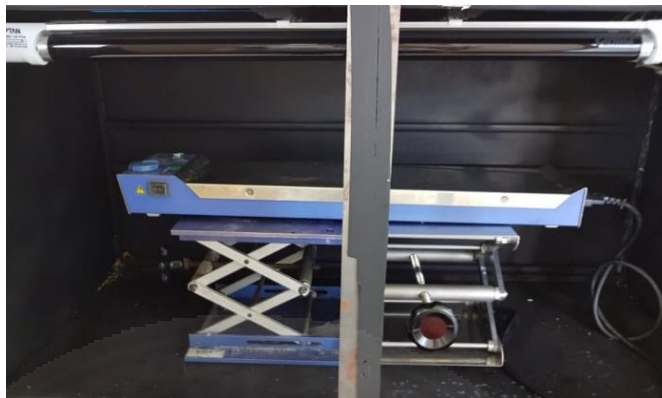
Figure 3.3 UV enclosure box for photocatalytic degradation of glyphosate
