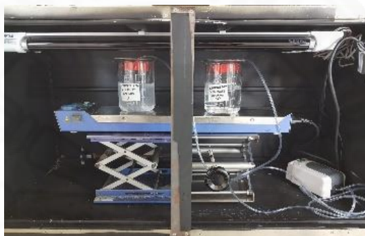
Figure 3.5 Photocatalytic degradation set-up for \text{TiO}_2 pellets
