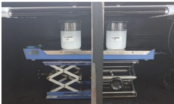
Figure 3.6 Photocatalytic degradation set-up of TiO 2 powder
