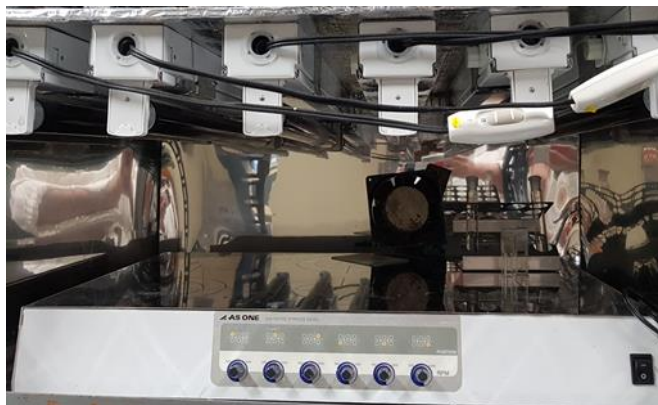
Figure 3.2 UV enclosure box for photocatalytic degradation of MB
