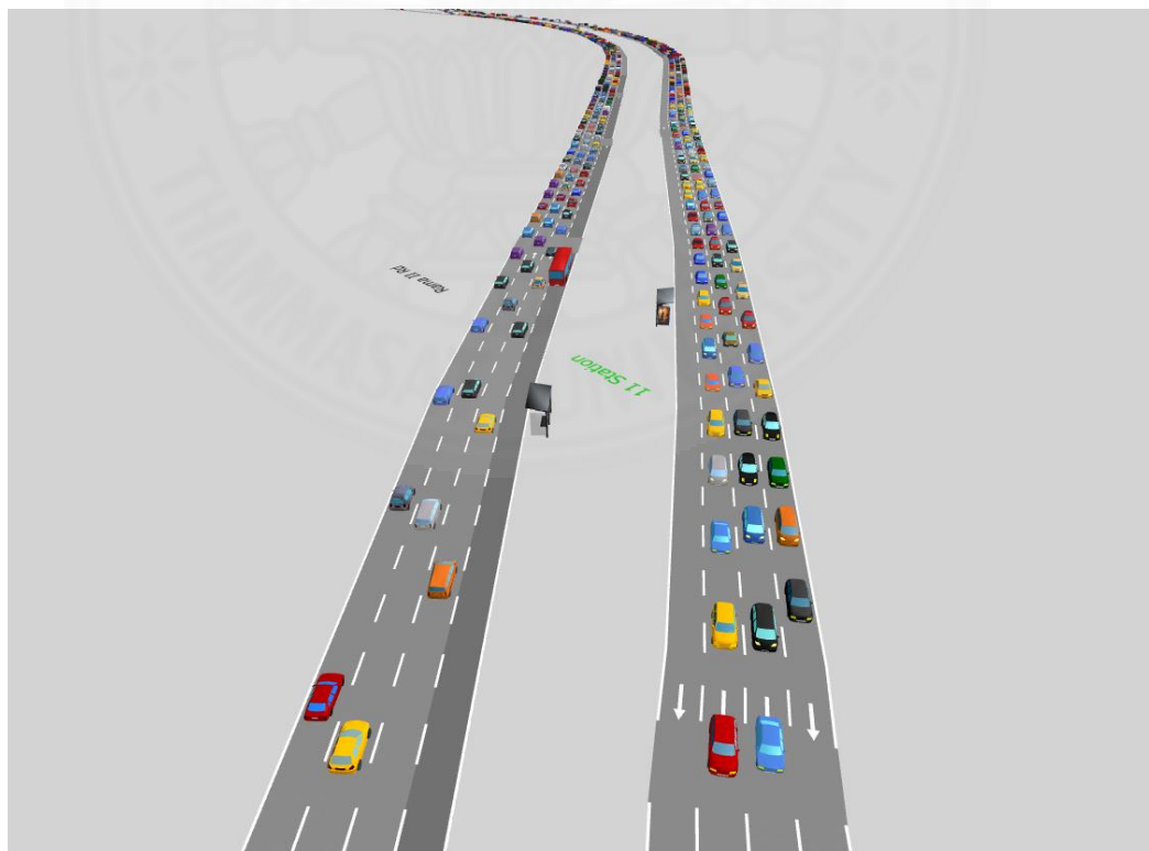
Figure 4.21 Traffic Simulation by Enforcing Fully Segregated Lane Solution in the Evening Peak Hours at Rama III Road
