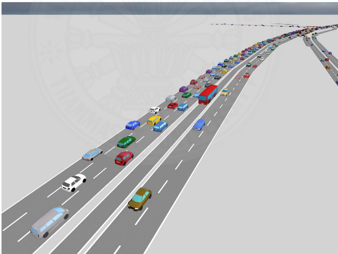
Figure 4.24 Traffic Simulation by Adopting Reversed Lane Solution in the Morning Peak Hours at Rama III Bridge
