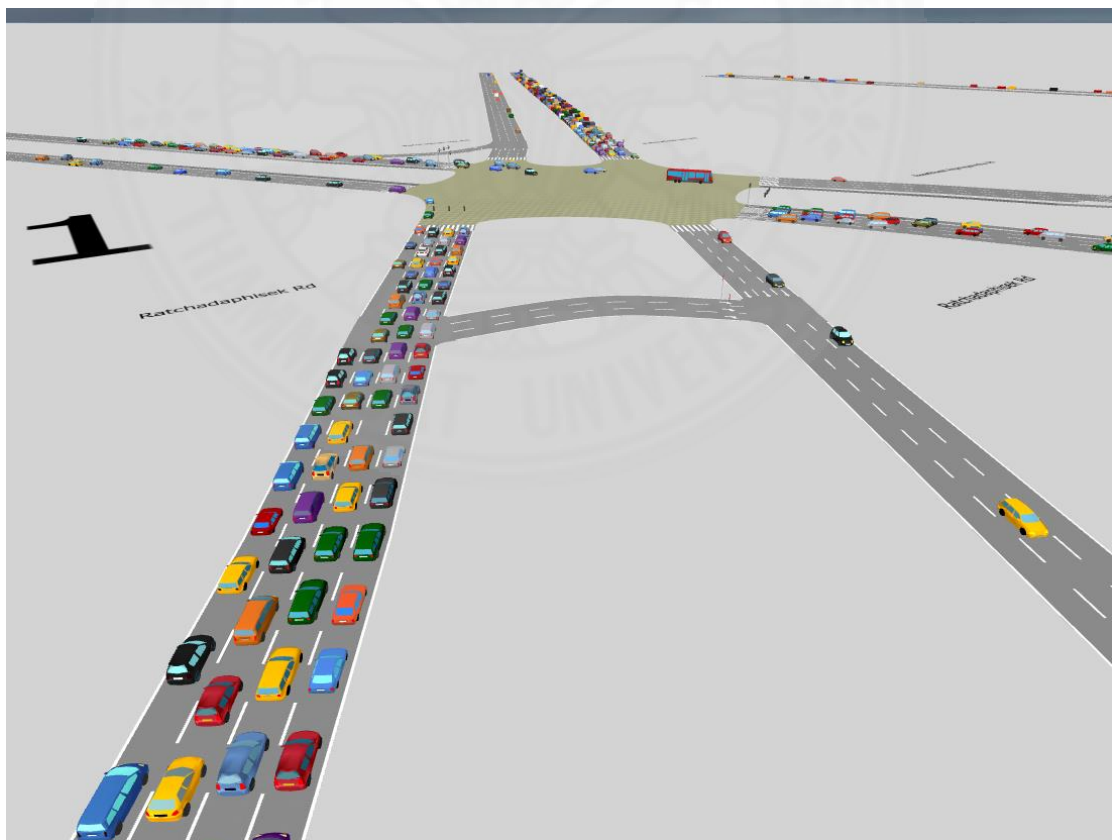
Figure 4.15 Traffic Simulation by Applying TSP Solution in the Evening Peak Hours at Narathiwat-Ratchadaphisek Intersection
