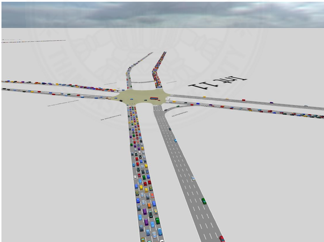
Figure 4.12 Traffic Simulation by Applying TSP Solution in the Morning Peak Hours at Narathiwat-Ratchadaphisek Intersection
