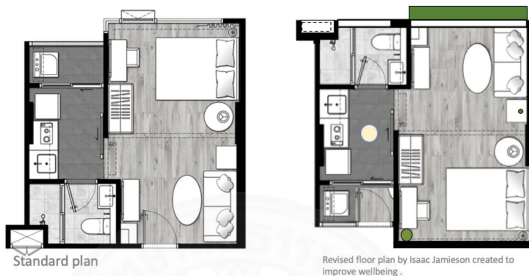
Figure 2.22 Standard and revised floor plan, indicating how design layout can be used to help optimize light exposures and biological functioning
