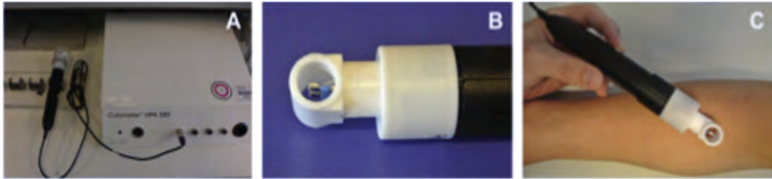
Figure 2.11 (A) Tewameter TM300 probe as part of the Cutometer MPA 580 (Courage & Khazaka GmbH, Cologne, Germany). (B) Tewameter sensors in probe head. (C) Probe positioning on the right lower arm. (55)
