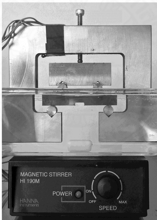
Fig. 2-4 Illustrations of stress corrosion cracking experiment.
