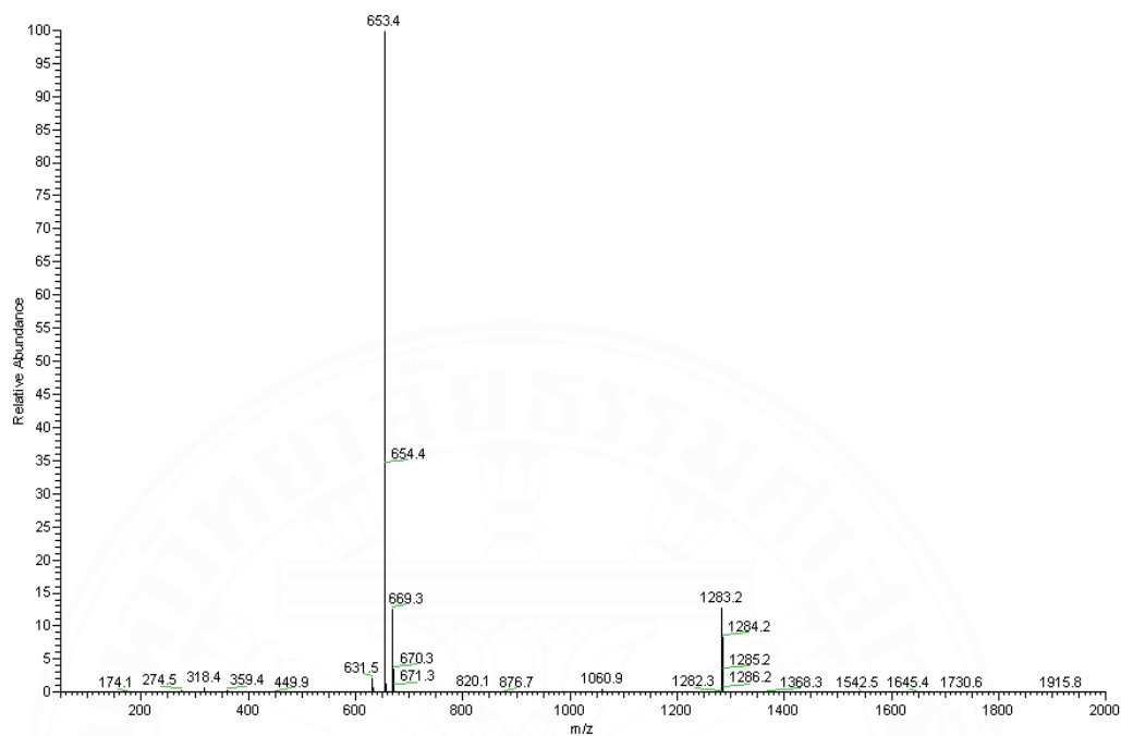
Figure D3 Positive mode mass spectrum of N,N' -diamino-bis(Fmoc-argenyl(Pbf)-glycyl)pimelic acid) ( 4 ) Found 654.4 [M+K]^+ , 670.3 [M+CH_3OH+Na]^+ , 1283.2 [2M+CH_3OH+Na]^+ ; Calculated fragment 616.32 [M]^+
