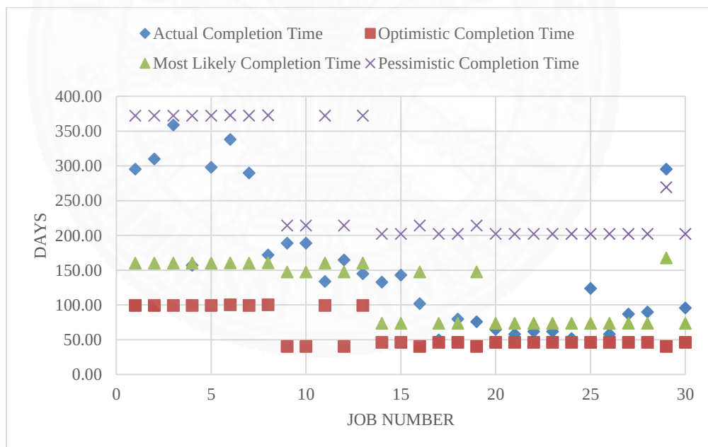
Figure 5.4 Planned Fuzzy Completion Times of Overhauled Jobs of fuzzy PERT /CPM Methods.
