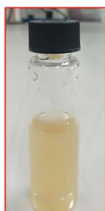
Acid treated 30h at 60°C
